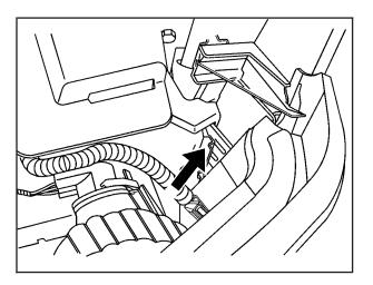
2. Press the retainer clip (arrow), located behind the turn signal housing, towards the outside of the vehicle.
